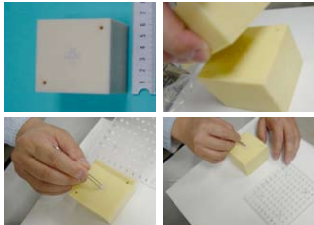
▲Radiotherapy Dosimetry Audit Device Designed by INER (including solid phantom and TLDS)
