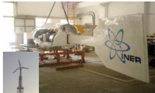
▲The INER-C25 Commercial Type WT and the Field Test Truss Tower
