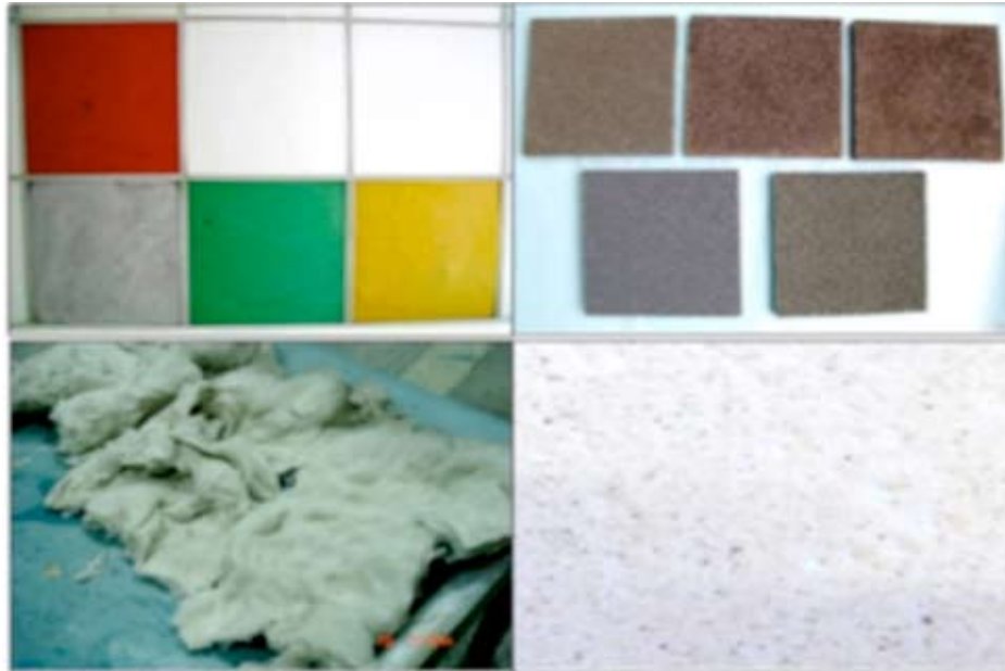
▲Recycled Products from Plasma Molten Slag(Top left: Colored light-weight slag plate; Top right: Soundproof slag plate; Bottom left: Slag fibers; Bottom right: Slag-fiber-containing non-woven paper)
