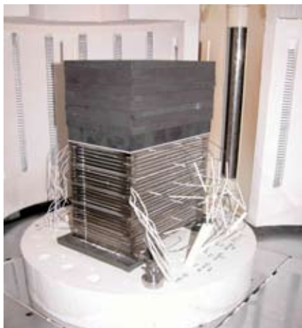
▲(a) The Outlook and (b) I-V-P Curves for a 25-cell Stack
