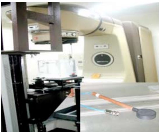
▲Primary Standard of the Absorbed Dose to Water for ^{60}\text{Co} and the Graphite Pancake Ionization Chamber
