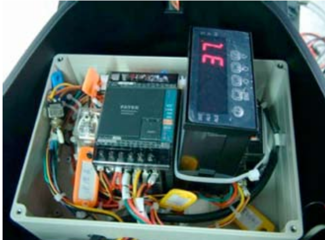
▲Integrating Control Unit of Engine Speed and Reformer Temperature
